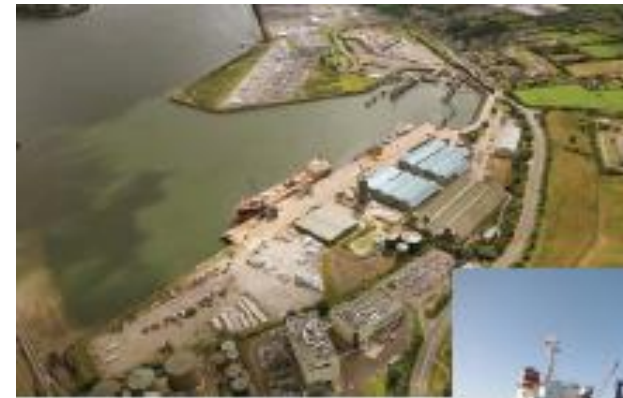
Ringaskiddy Deepwater Berth Berth Length 485m Depth 13.4m Storage Spaces behind berth 10ha
